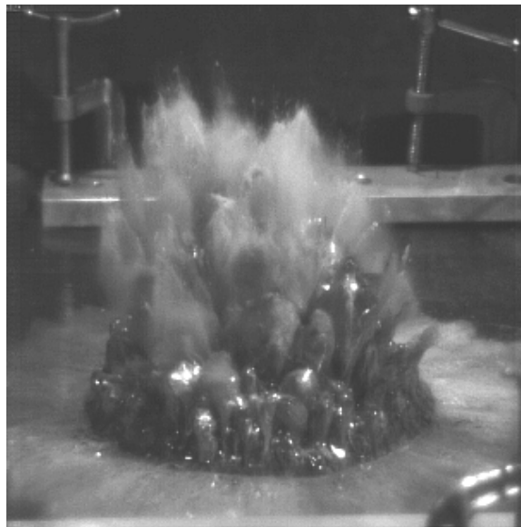
Figure 5.8: Interaction of upward moving soil from a shallow buried explosive with a clear rubber sheet.
