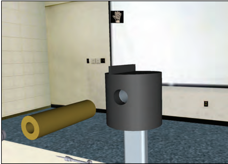
Plate 9: An example of subtype B4 symmetry where the pin can be inserted from two different positions (either side of the piston hole). For each position either the alternate or the primary orientation around the secondary axis may be used.
