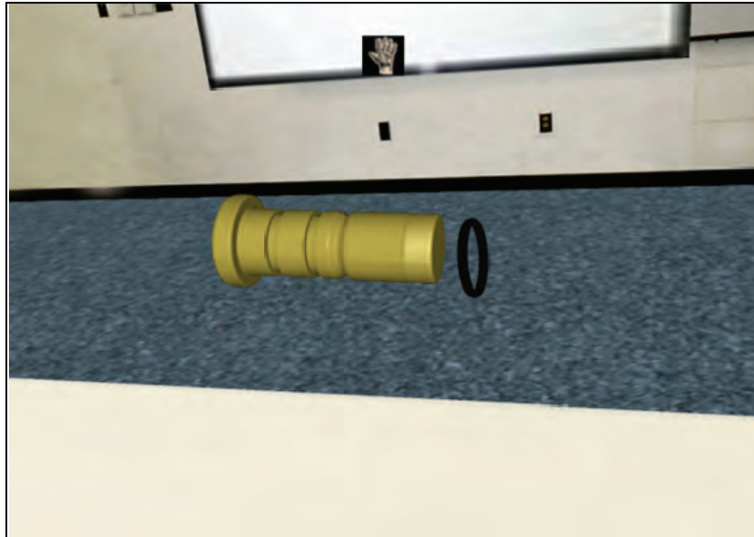
Plate 15: Rubber o-ring must be rolled on top of the rightmost rectangular groove.
