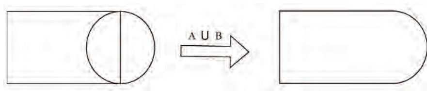
Figure 4.7: Union of two primitive solids
