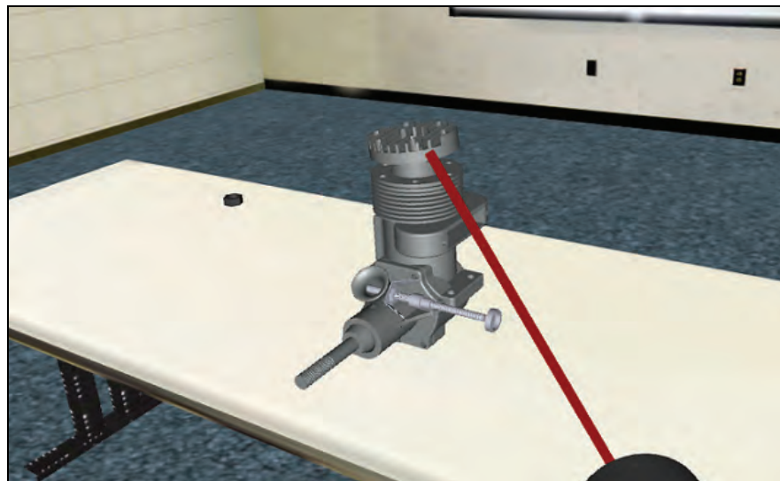
Plate 6: Virtual demonstration of attachment of engine cover to top of engine case
