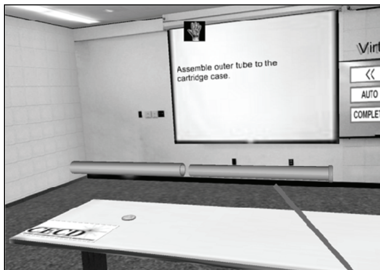
Figure 8.3: An example of sub-type B2 symmetry where the attachable part (outer tube) can only be inserted at the primary position, but with either primary or alternate orientation (around the secondary axis). Secondary axis is perpendicular to the main axis, which is the axis of the cylinder.
